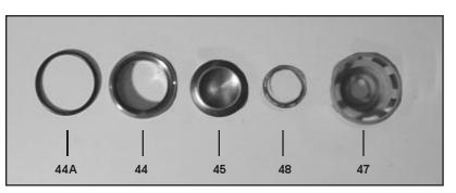
2. To disassemble the valve, screw the bolt into the retainer until the valve plate (45) presses the valve seat (44) out of the spring retainer. Examine all parts and replace if necessary. If the seat doesn't come out, use a valve puller to remove.
